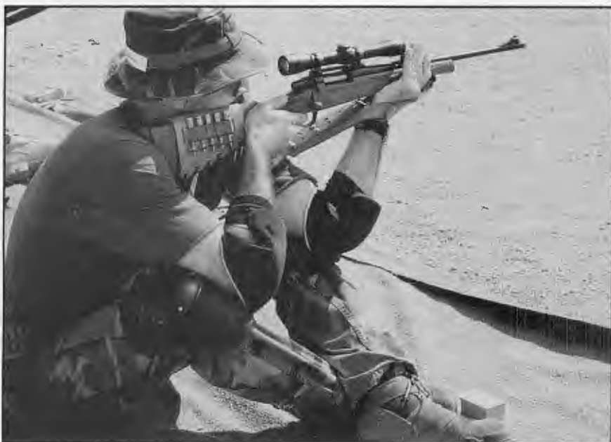
Gabe Suarez, who serves with a major California law enforcement agency, fires his Remington Model Seven .308 Winchester caliber rifle from the sitting position. This short-action design, introduced in 1983, has an 18.5-inch barrel and a walnut stock with a modified schnabel fore-end.
